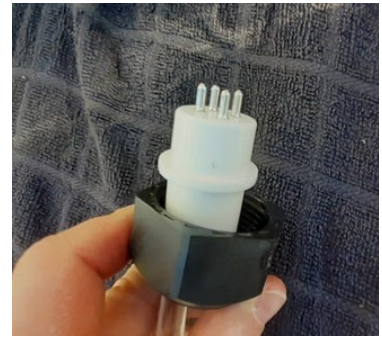
Slide threaded cap over lamp.
